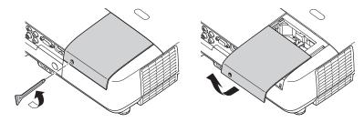
4. Loosen the two screws holding the lamp in place (you can't remove them).
