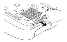
3. Slide the new air filter into the slot until it clicks into place.
