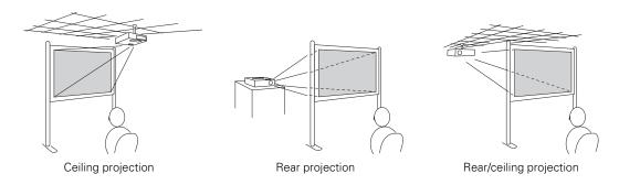
To project from overhead, you'll need the optional ceiling mounting hardware (see page 11). You'll also need to select the appropriate **Projection** setting in the projector's Extended menu to orient the image correctly (see page 50).
