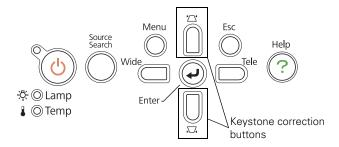
■ Select the **Keystone** setting in the projector's **Settings** menu (see page 49). Then use the arrow buttons on the remote control to adjust the shape of the image.
